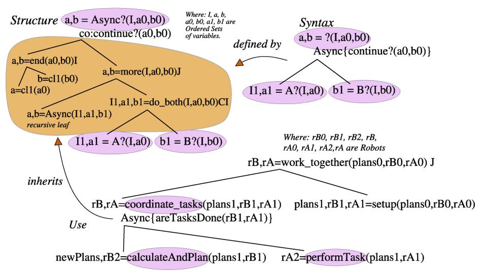
To understand Async's use at coordinate\_tasks, go to Async's definition and to understand do\_both go to CI's definition. Ultimately, coordinate\_tasks is defined in terms of the Join, Include and Or primitive control structures.
