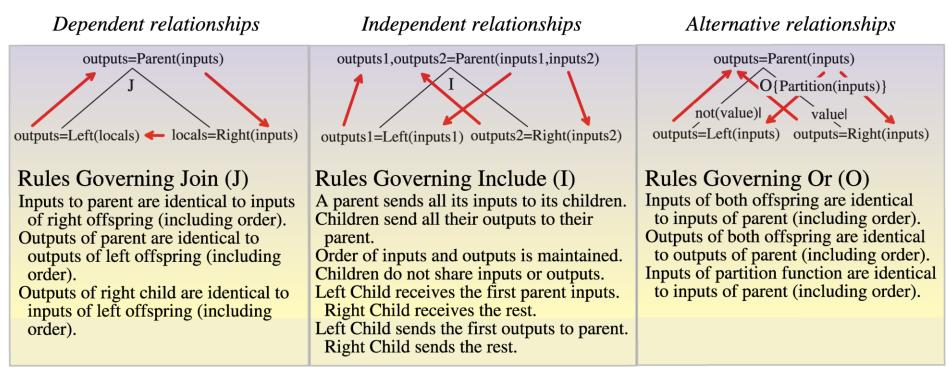
Where: inputs, locals, outputs, inputs1, inputs2, outputs1 and outputs2 are Ordered Sets of variables. In the Include structure, the Left child is a higher priority than the Right child; and the leftmost output variable is the highest priority variable.
